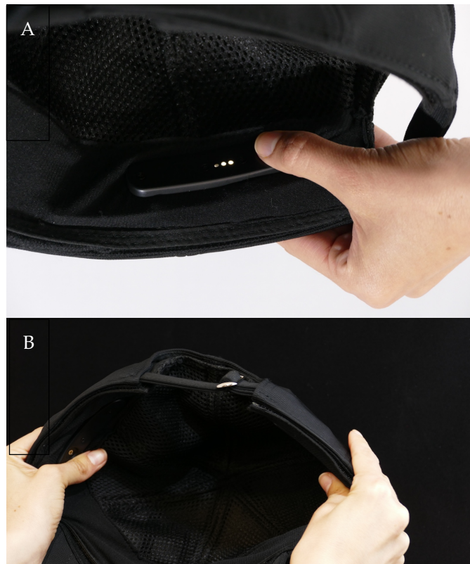
Figure 2: A- The StimuField Cap includes an interface element featuring the single power button and LED indicators that provide information about the charge level. The interior includes a removable, washable inner liner made from breathable materials, allowing the user to clean the portion that comes into contact with the scalp. B- The StimuField Cap incorporates a flexible inner core and an adjustable back strap for a comfortable, adaptive fit. It also includes a magnetic charging port for easy and secure power connection.
